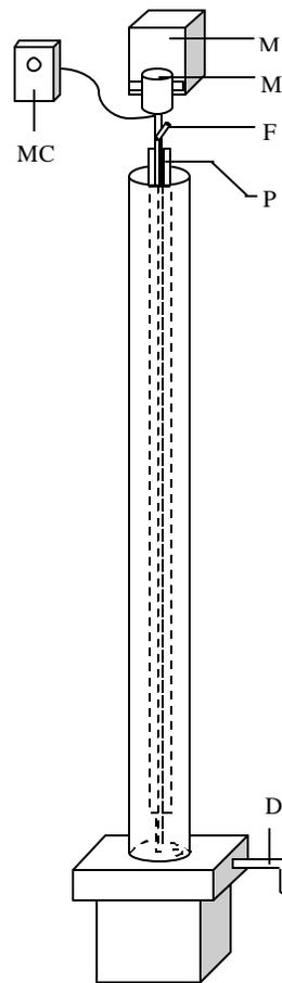
Figure 2. Side view of the clear stream tube (water depth, 300 cm; diameter 15 cm) used to determine swimming height above the bottom of pallid sturgeon free embryos and larvae. Key to components: M = motor, MM = motor mount, MC = motor control, F = fish introduction tube, P = paddlewheel, and D = drain. The rotating paddlewheel created a water current circling the tube at a velocity of 2 cm/s.
